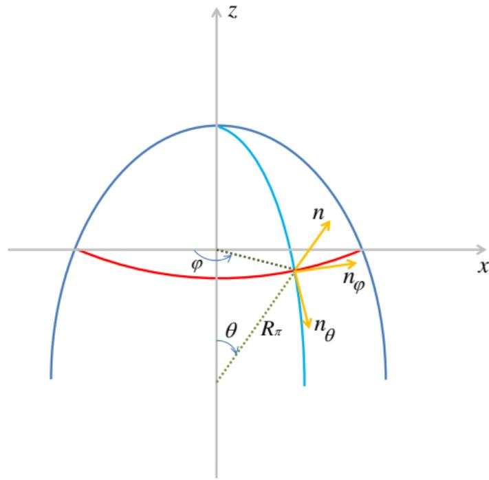
Shell Element is cut out by two meridians and two parallels
