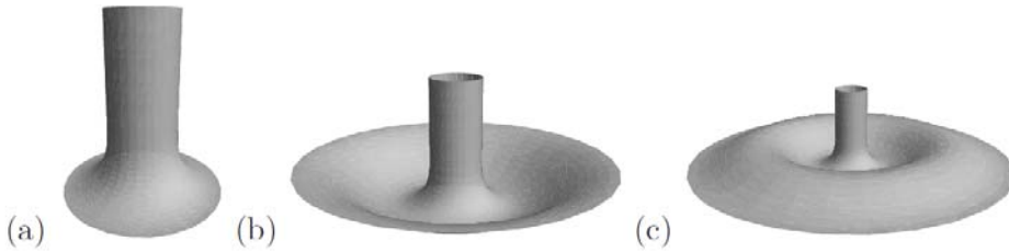
Figure 4. Profile curves and the corresponding junctions between a carbon nanotube and a flat graphene sheet with parameters \lambda = 1 and \mu_1 = 0 . The length of the profile curve is: (a) L = 2.053 ; (b) L = 5.043 ; (c) L = 8.076 .
