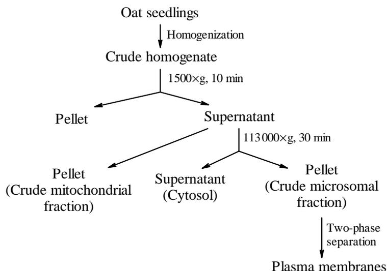
**Fig. 1.** The scheme of subcellular fractionation of plant material.
