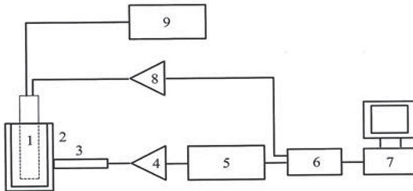
Fig. 1. Thermoluminescence (TL) set-up: 1 – sample holder; 2 – Dewar flask with liquid nitrogen; 3 – photomultiplier tube; 4 – amplifier; 5 – photon-counting device; 6 – ADC plate; 7 – PC; 8 – bridge amplifier; 9 – transformer.
