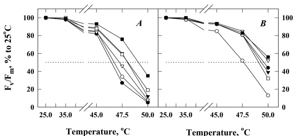
**Fig. 6.** Temperature dependence of relative variable fluorescence ( $F_v/F_m$ ) in leaf discs from bean plants subjected to different acclimation procedures. The conditions of acclimation and measurement procedures as well as the curves symbols are as in Fig. 4. Data are presented in percent to  $F_v/F_m$  value measured at 25°C
