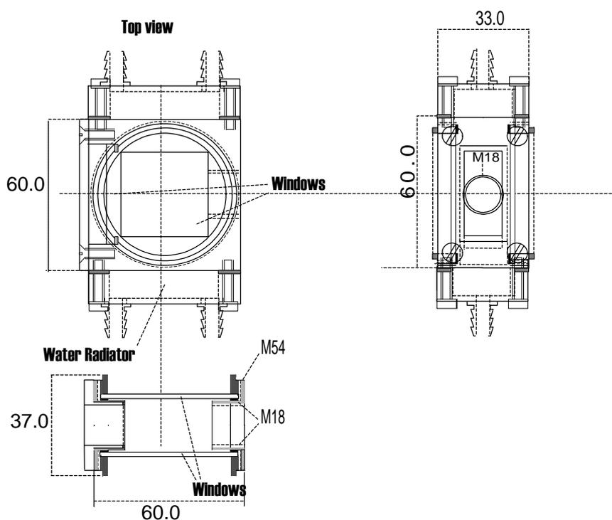
Fig. 3. Detailed diagram of the polarographic cuvette.
