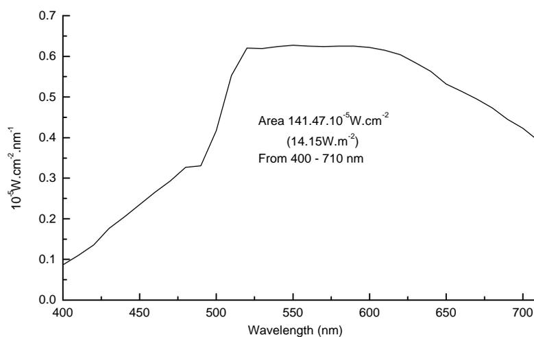
Fig. 7. Spectral distribution of the irradiance energy at halogen lamp – 100 W/12 V.
