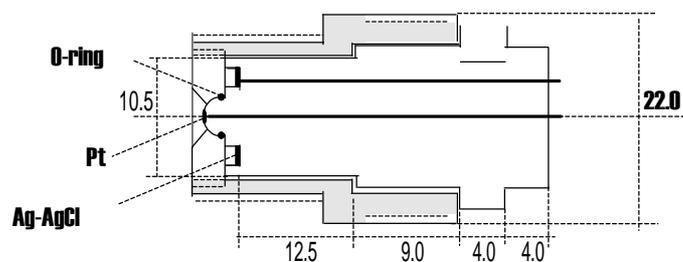
Fig. 4. Polarographic oxygen electrode.
