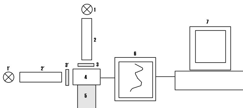
**Fig. 2.** Experimental set-up for quantum efficiency investigations. 1 and 1' – halogen lamps (100 W/12 V); 2 and 2' – collimators; 3 and 3' – interference filters (650 nm); 4 – polarographic cuvette with oxygen electrode; 5 – magnetic stirrer; 6 – polarograph (OH-105, Radelkis, Hungary); 7 – IBM compatible computer.
