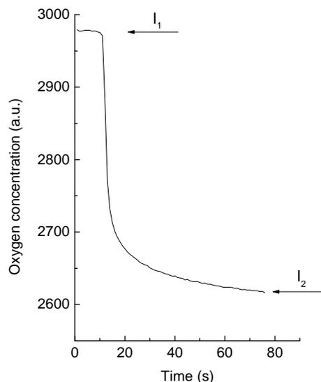
**Fig. 5.** The calibration record of the polarographic oxygen electrode.  $I_1$  – polarographic current for distilled water saturated with atmospheric oxygen ( $0.276 \mu\text{mol O}_2/\text{ml}$ ) and  $I_2$  current after addition of the several crystals of dithionite. Polarograph sensitivity –  $10^{-7} \text{ A/Div}$ .
