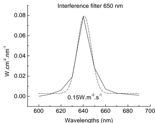
**Fig. 8.** Spectral distribution of the energy after the 650 nm interference filter (solid line) and a Gauss function approximation (dashed line).
